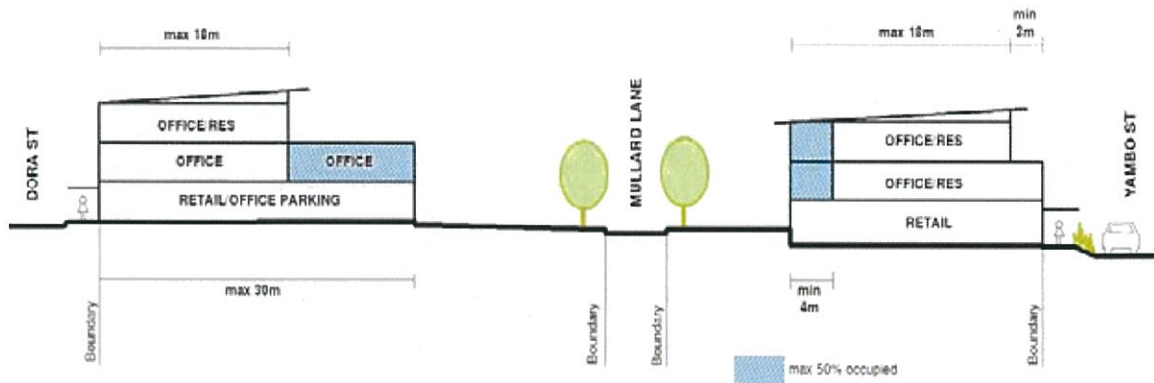
Figure 14: Block A Section A-A
